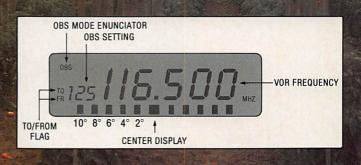
The all new, HT 870 NAV/COM is a microprocessor controlled, **navigation capable**, 760 channel COM transceiver and 200 channel NAV receiver. The HT 870 features a **built-in CDI** (Course Deviation Indicator), **quick change**, rechargeable NiCAD battery pack and as an option a **spare alkaline battery pack**.
