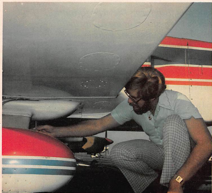
Four fuel sump drains on the Tiger are checked with a special fuel sampler cup.
