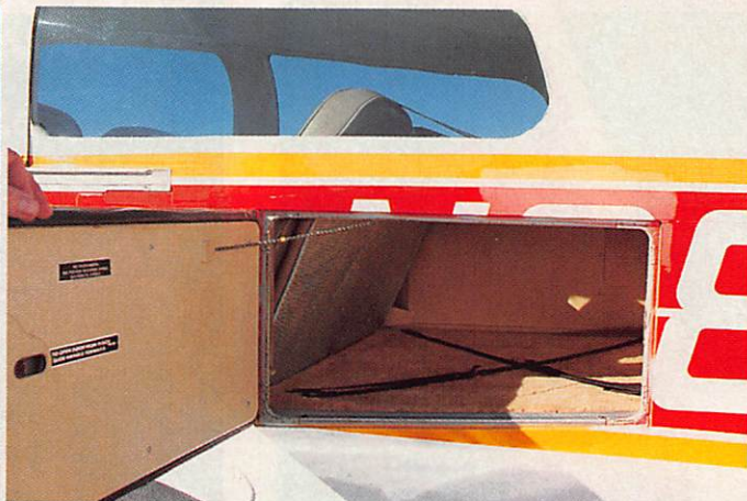
Nancy Clinton's Tiger shows the hallmarks of the breed: sliding canopy, "mail slot" baggage door, and ancillary controls on the center console.
