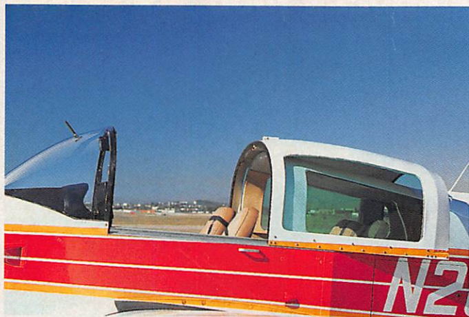
Nancy Clinton's Tiger shows the hallmarks of the breed: sliding canopy, "mail slot" baggage door, and ancillary controls on the center console.
