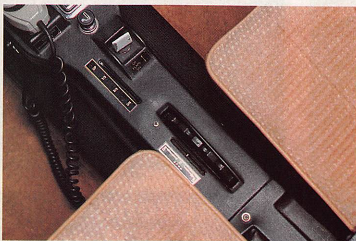
Nancy Clinton's Tiger shows the hallmarks of the breed: sliding canopy, "mail slot" baggage door, and ancillary controls on the center console.
