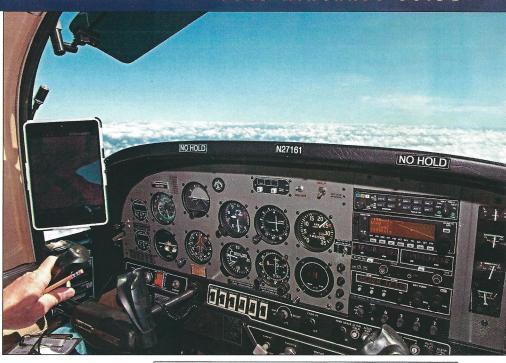
A single radio stack works for basic IFR avionics in a Cheetah, top. Panels in later Tigers look slightly more modern, middle. Garmin's G1000 was standard in the last of Tiger Aircraft's AG-5Bs, bottom.
