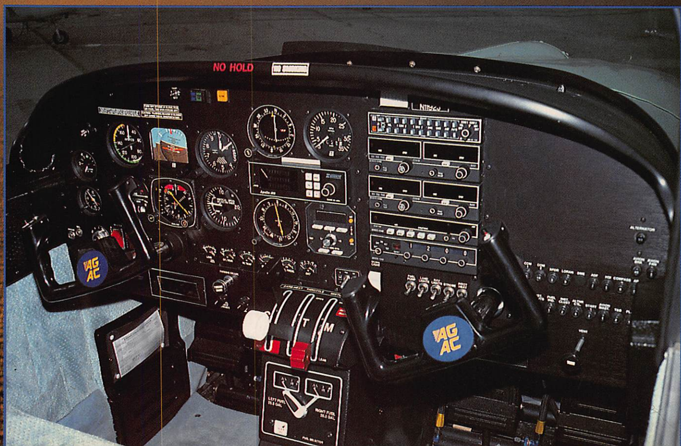
TOP: Flywriter Bill Cox says "It's unquestionably the most agile, non-aerobatic production airplane available in the United States and a sheer delight to fly." BOTTOM: For 1992, the Tiger's panel is all-metal and all-electric, a far cry from the original fiberglass panel of the '70s. The all-King stack includes KX 155 radios, transponder and ADF.
