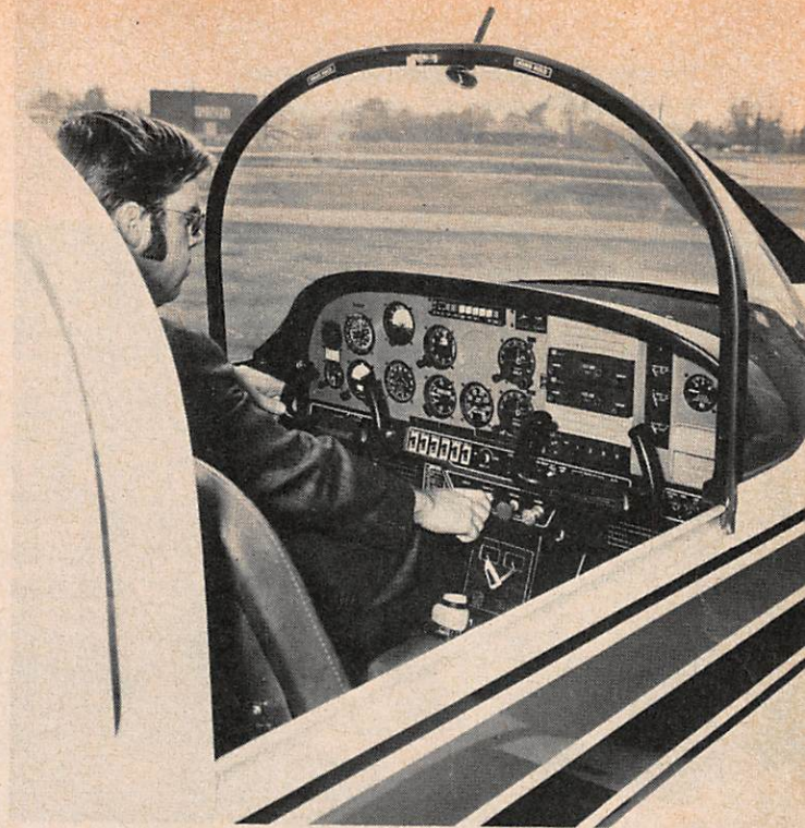
RIGHT—Sliding canopy gives the Tiger an open-cockpit touch. Performance increase of new model is substantial. BELOW—Inflight shot of panel shows easy IFR descent at 60-mph IAS, using full aft trim and 90 rpm for 600 fpm! OPPOSITE PAGE—Nose-to-nose are the Tiger and the famous TR-2. Two beautiful planes that are hard to beat.
