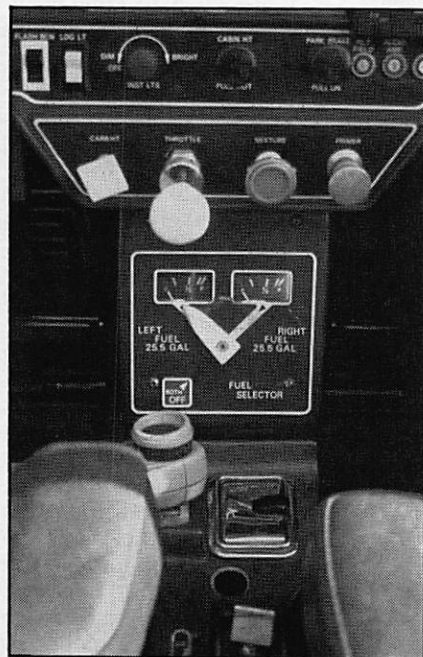
Detail of the fuel selector switch at front of center console. Note ashtray on console.
