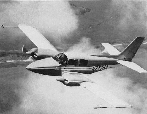
and climb capability. The whole package perches high on slim gear that retract conventionally inboard (mains) and forward (nosewheel). (There was some talk of folding the mains toward the tips ala Me-109 to allow more room for fuel in the inboard wings, but that seems unlikely this late in the game.)
